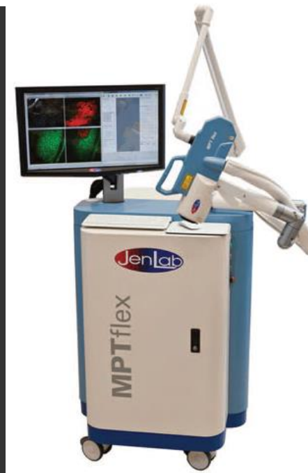
Figure 3. Multiphoton hybrid tomograph MPT-CARS for lipid/water imaging by CARS, detection of NAD(P)H, flavins, keratin, elastin and melanin by two-photon autofluorescence as well as collagen imaging by SHG. 27,28
