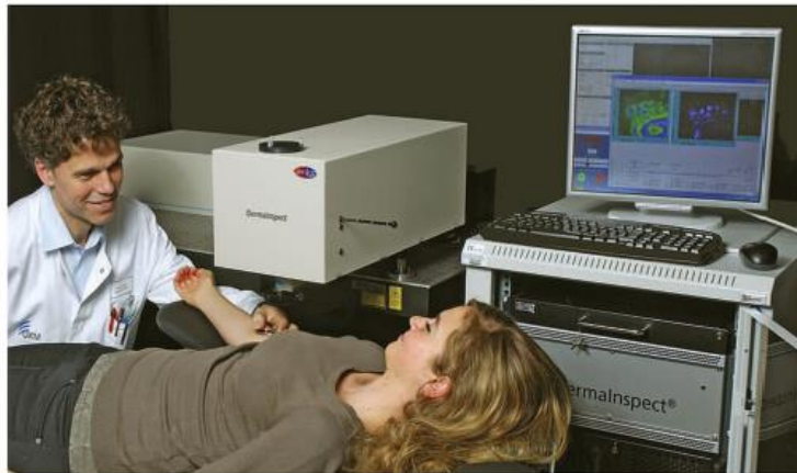
Figure 2. Multiphoton-tomograph Dermalmspect™ at the University of Münster, Germany. The 3D imaging system can be expanded to a 5D tomograph by adding a spectral FLIM module.
